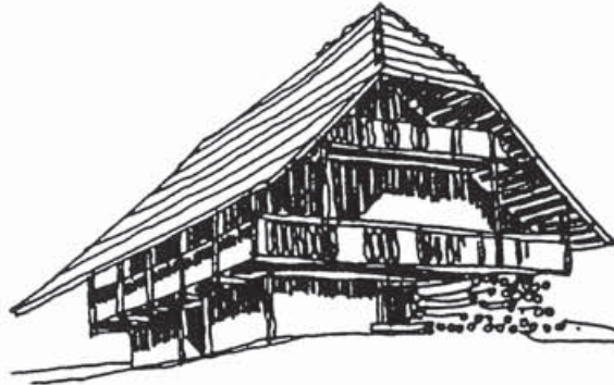
A typical (Bernese region) Alpine “Chalet.” Dwelling areas, cowshed, and barn are all grouped under a common roof. This reduces heat loss, offers protection for the balconies and working spaces, and shelters the facades from bad weather.
