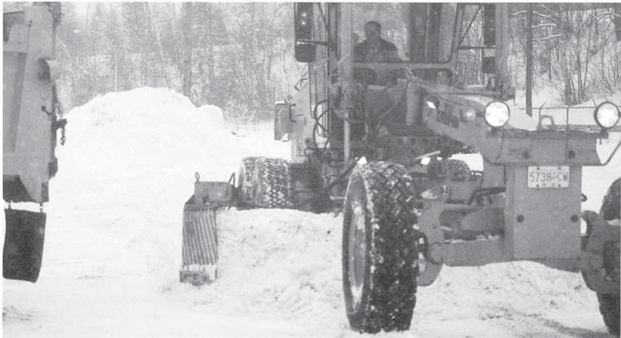
A grader equipped with a snow-gate is shown here with the gate in the "down" position. The gate is dropped to carry snow through the driveway opening. Snow is deposited on the far side of the driveway. Photo courtesy of the City of Prince George
