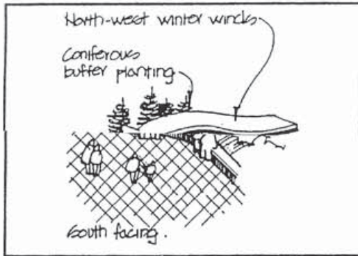
"Sun Pockets" and protected spaces are created by strategic landscaping (Source: Winter Cities Manual)
